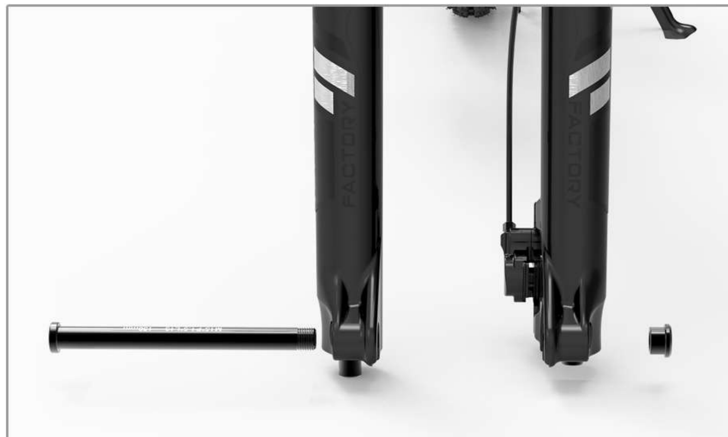
04 Remove the front wheel mounting shaft
