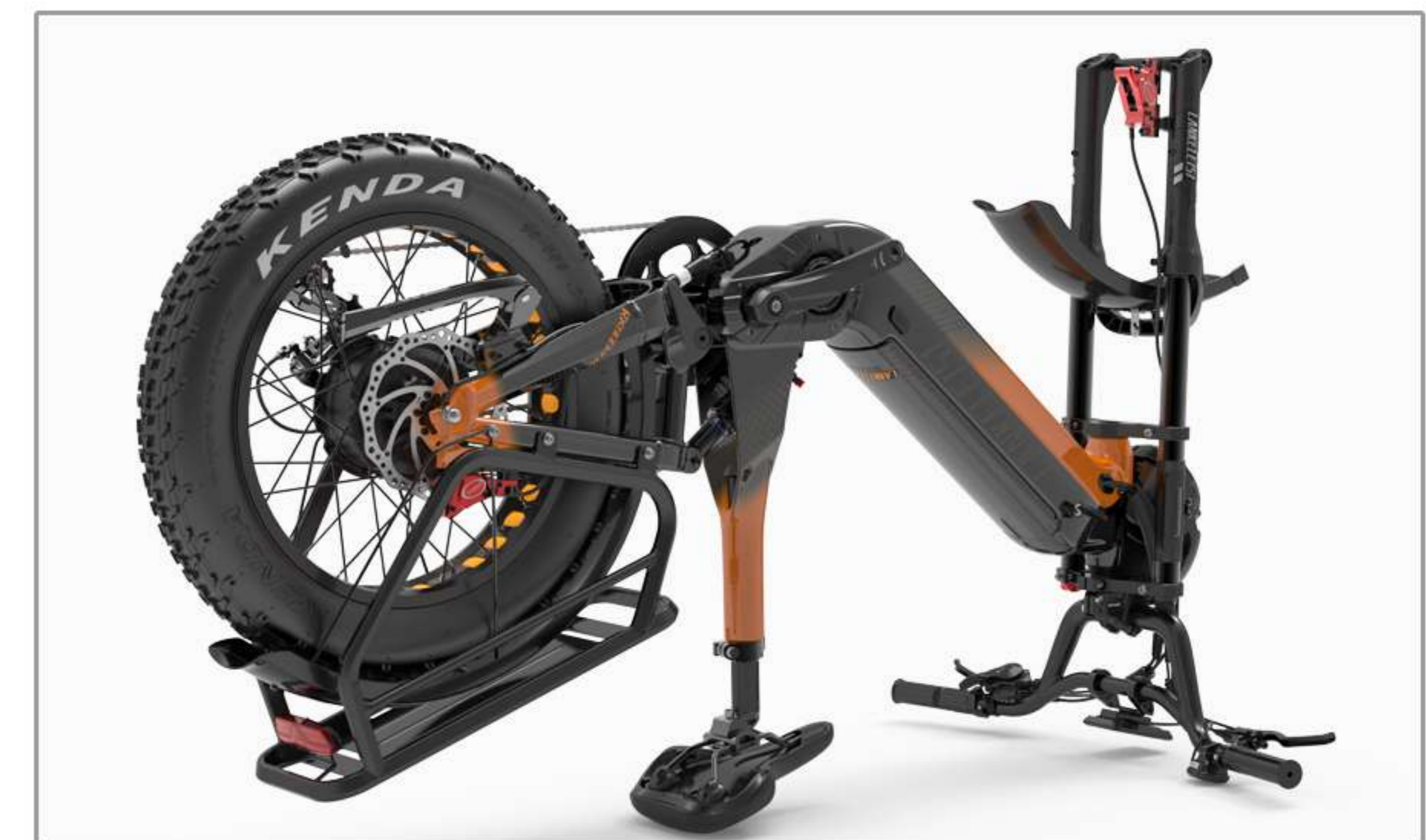
06 Preliminary work for installing front wheel Invert the entire vehicle
