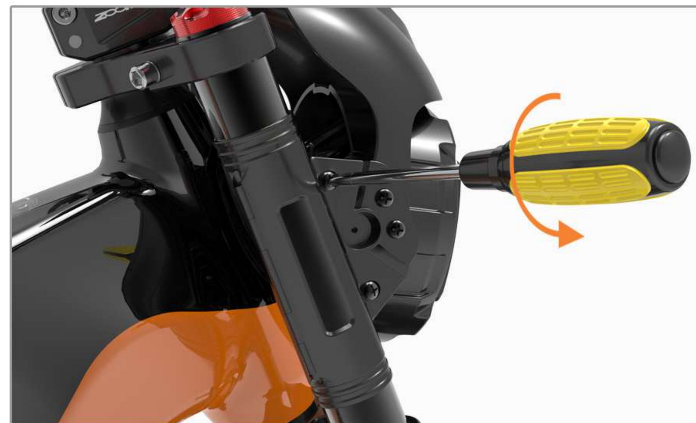
05 Locking screw, headlight installation completed
