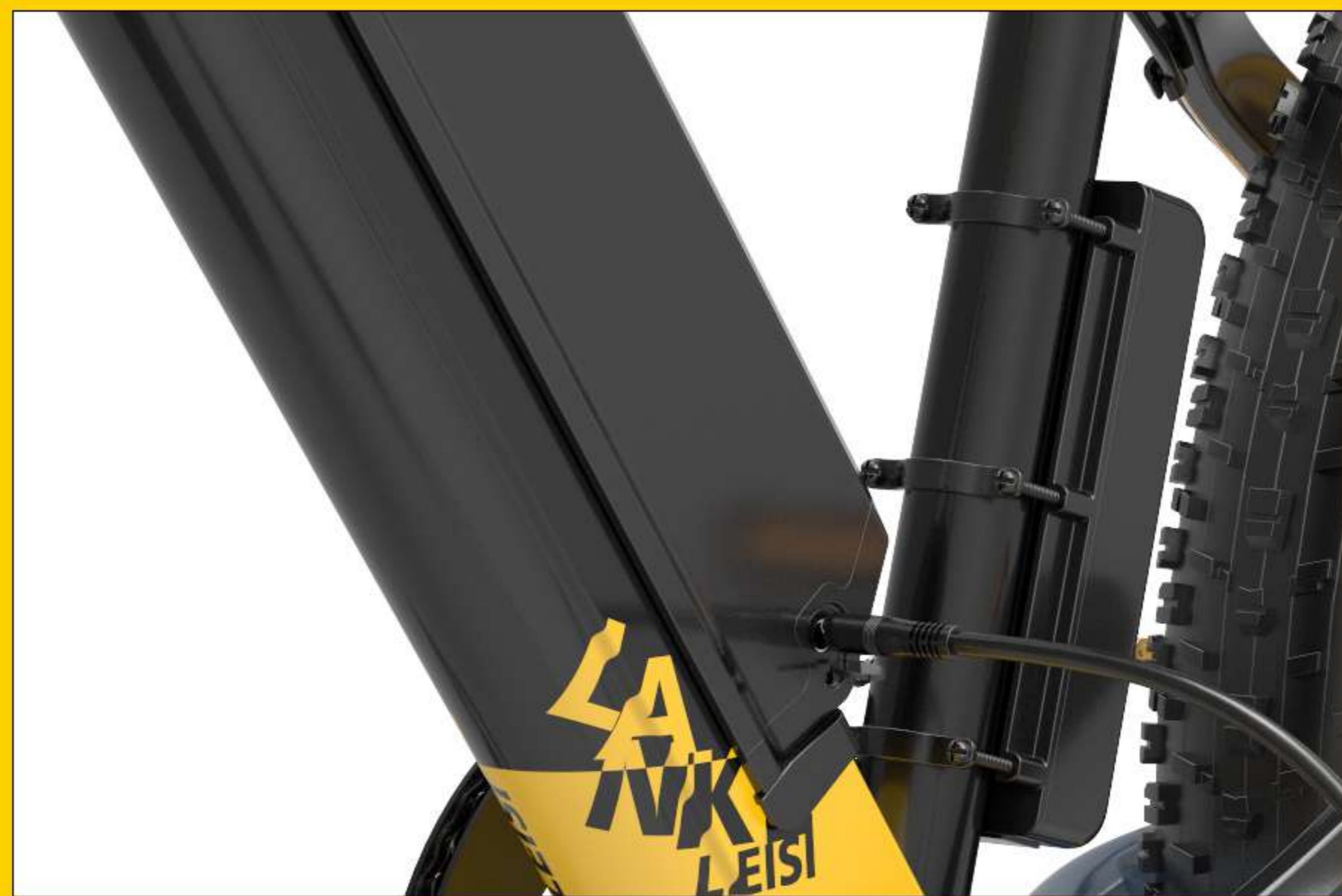
A. Recharge the battery on E-Bike directly
