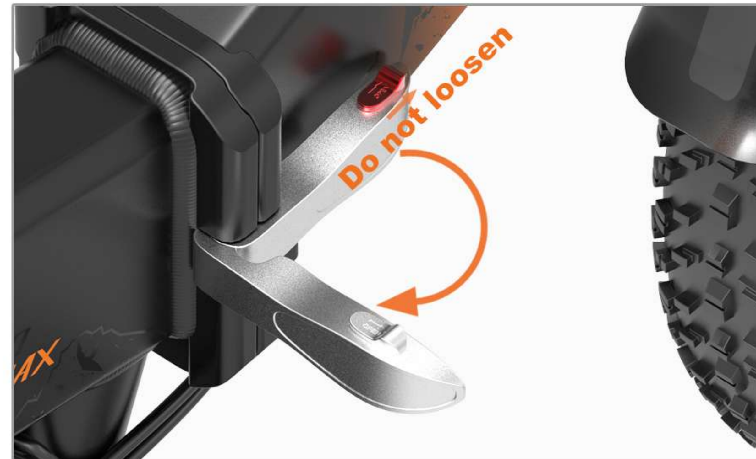
02 Do not loosen the safety buckle, use your hand to forcefully open the folding buckle
